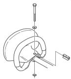
3 Now make a final adjustment to give yourself a comfortable working position. Tighten the screw. CAUTION! The loop handle and hand guard must not be fitted behind the arrow marked on the shaft.
